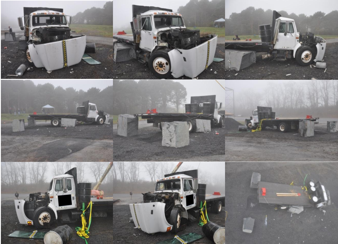
Figure 4-49. Post-test location and condition of the impact vehicle in BFT-2
