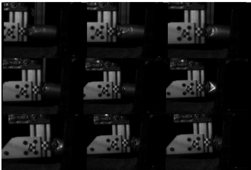
Figure 6-16. High-speed image sequence of dynamic crush test
