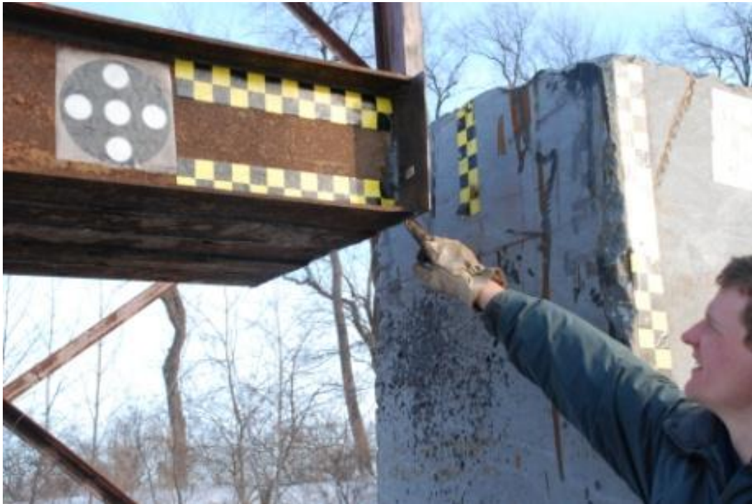
Figure 4-56. Post-test condition of impact sled after MFT-1
