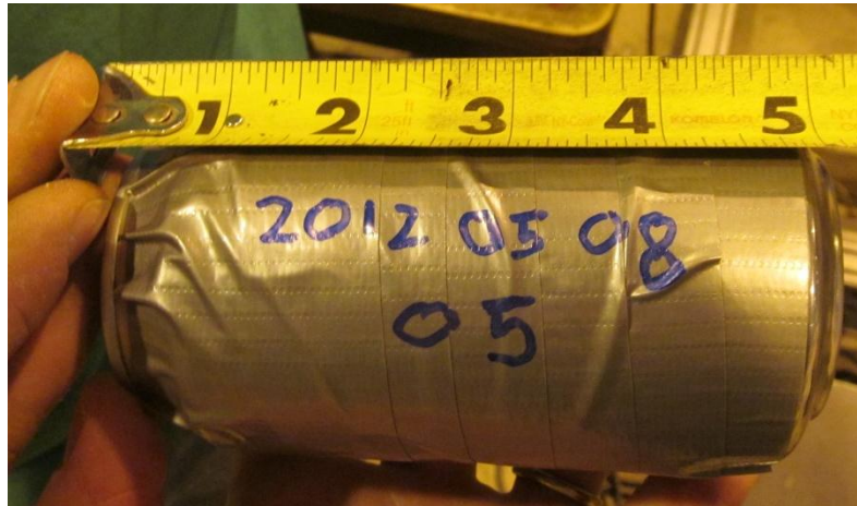
Figure 6-15. Typical spacing for duct tape wrappings
