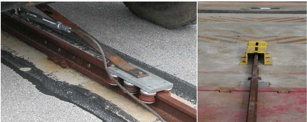
Figure 4-3. Full scale guidance system: bogey assembly (left) and bogey catch (right)
