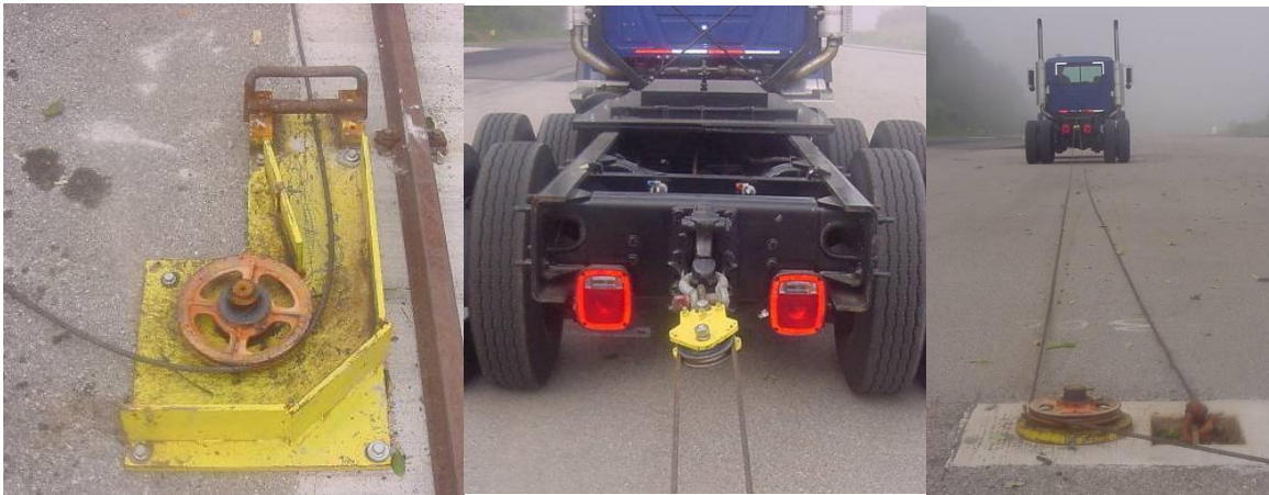
Figure 4-4. Full scale towing system: first re-directional pulley (left), speed multiplier (center), and second re-directional pulley (right)
