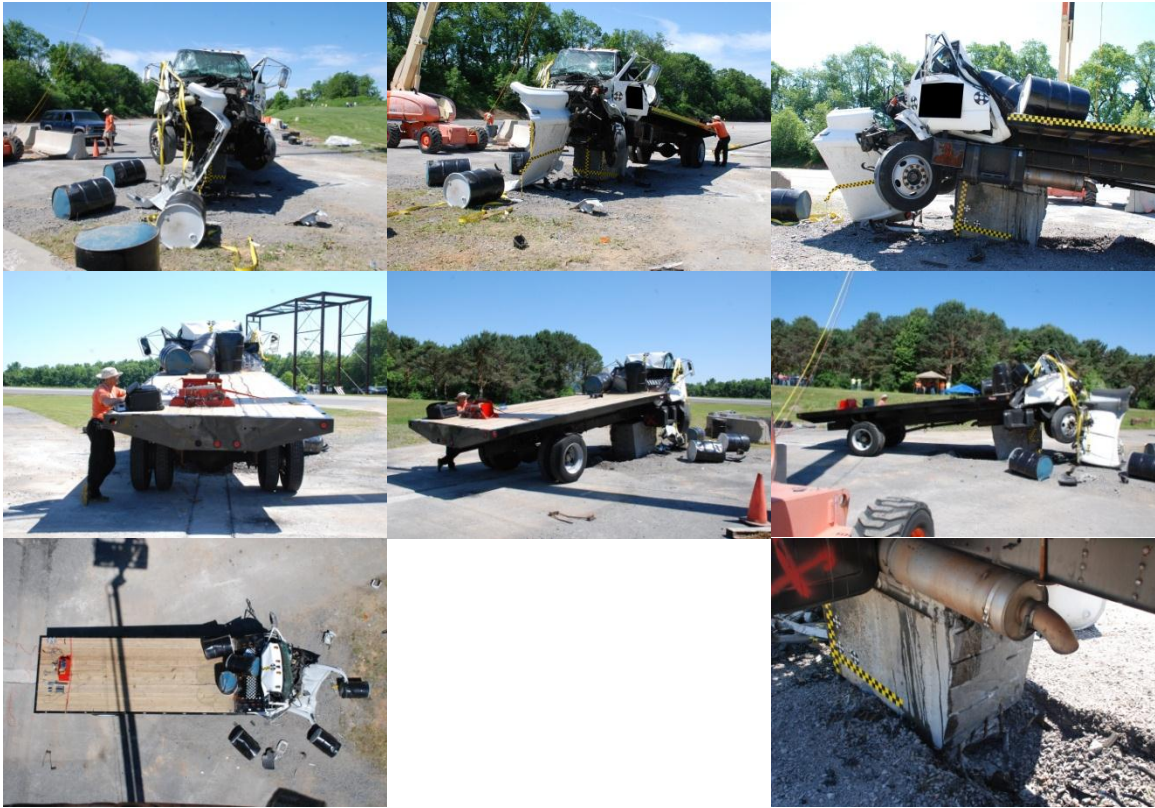
Figure 4-40. Post-test location and condition of the impact vehicle in BFT-1
