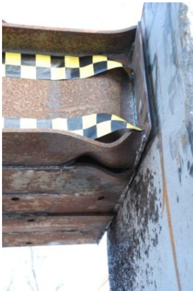
Figure 4-58. Post-test condition of impact sled after MFT-2
