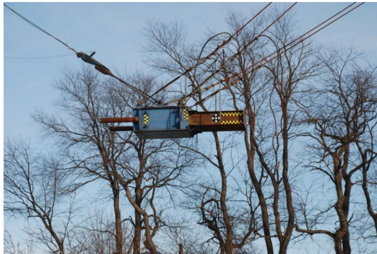
Figure 4-12. Impact sled with quick release mechanism
