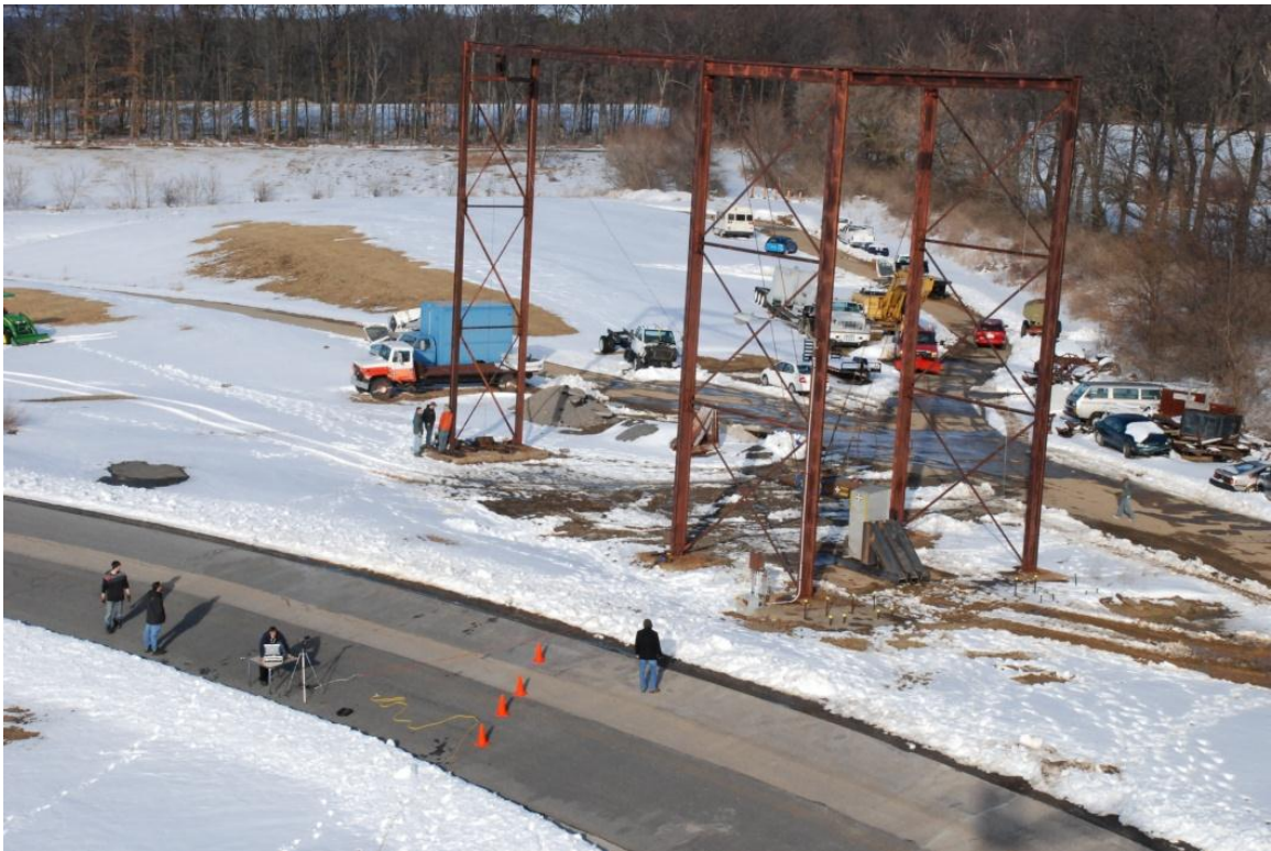
Figure 4-7. Crash Safety Research Institute medium scale impact pendulum
