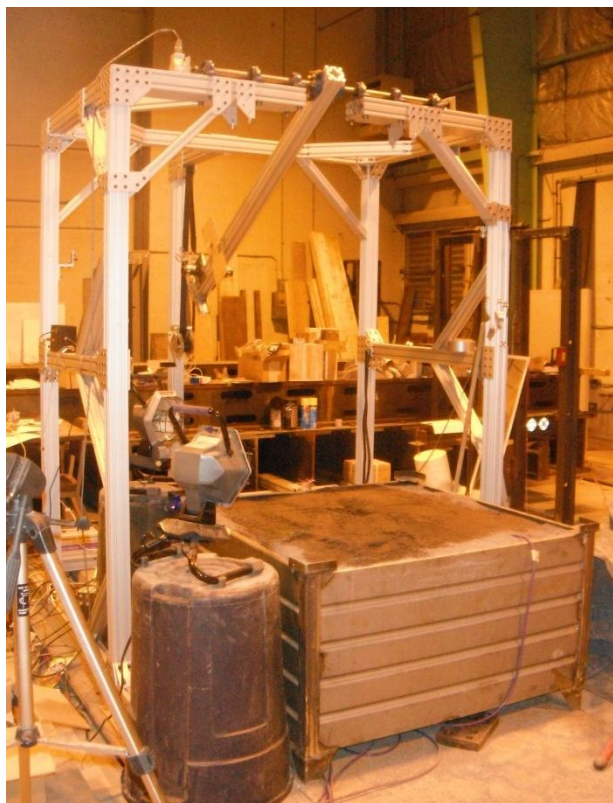
Figure 6-9. SSCR pendulum used in small scale testing of soil-fixed boulders
