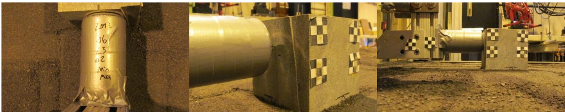
Figure 8-4. Pre-test conditions of the impact beam and crush material in SSMMBST-1
