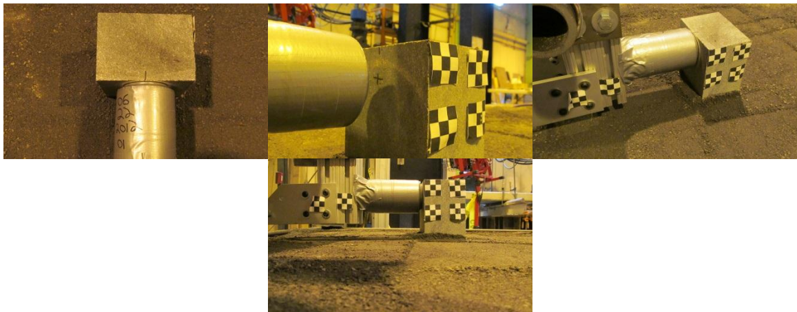
Figure 6-18. Pre-test conditions of the impact beam and crush material in SSBST-1
