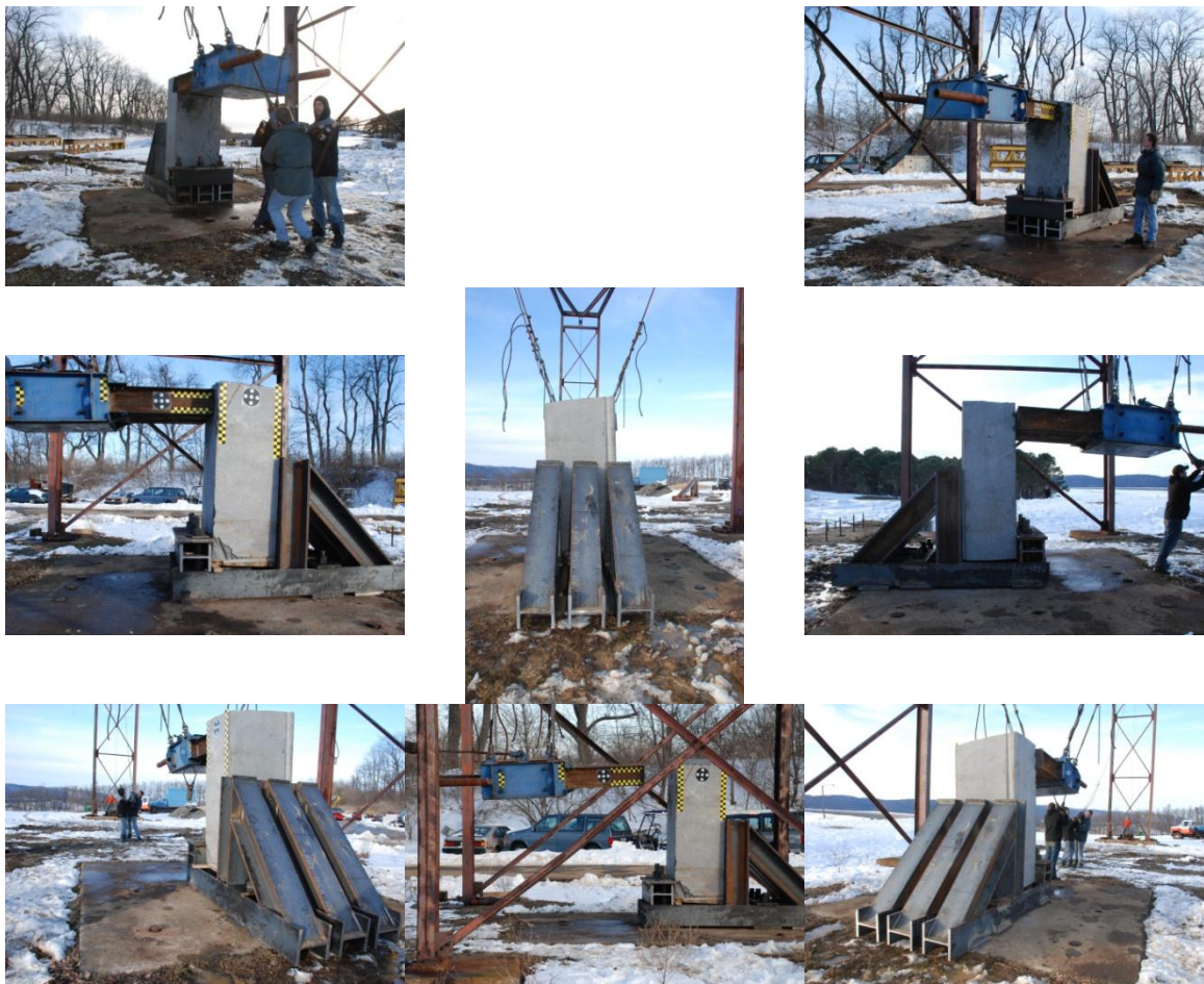
Figure 4-55. Post-test condition of ABG-01 after MFT-1
