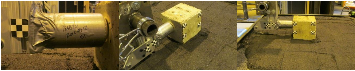
Figure 6-28. Pre-test conditions of the impact beam and crush material in SSBST-2
