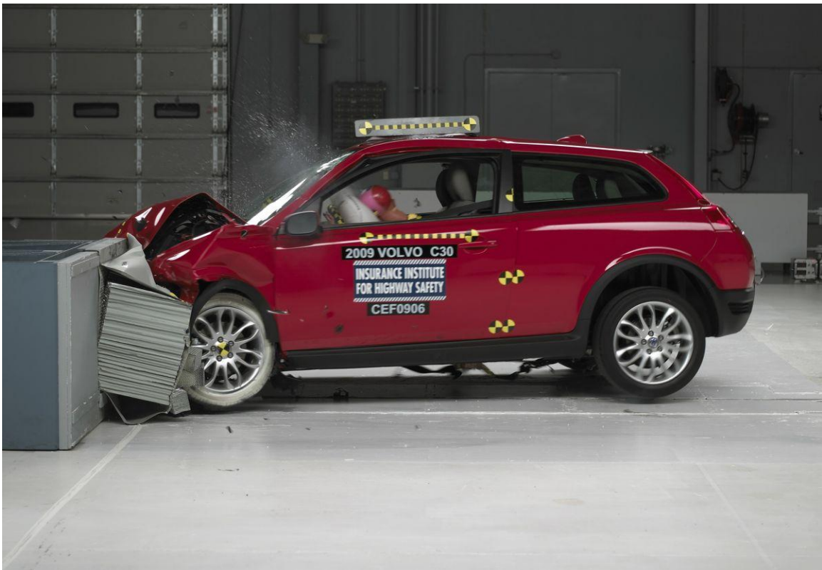
Figure 1-1. 31 mph crash test of a 2009 Volvo C30 into a rigid wall [3]
