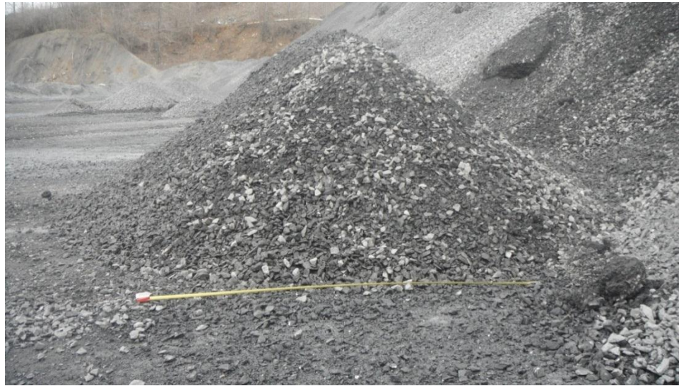
Figure 4-5. Modified 2A limestone gravel in loose state
