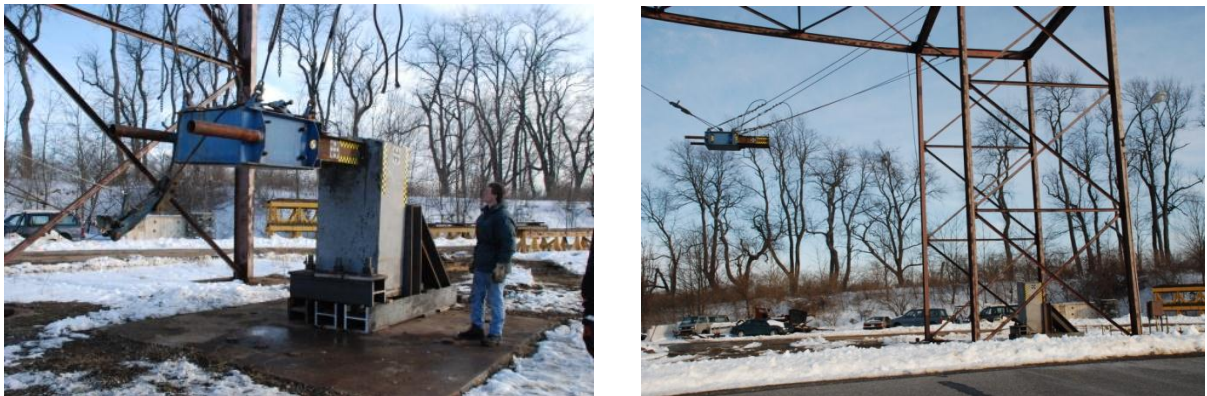
Figure 4-13. Example of the change in elevation of the impact sled; equilibrium position (left) and desired elevation change (right)
