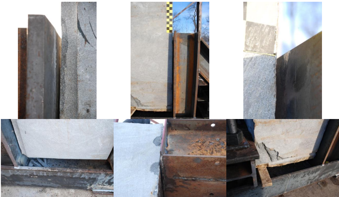
Figure 4-57. Post-test condition of ABG-01 after MFT-2
