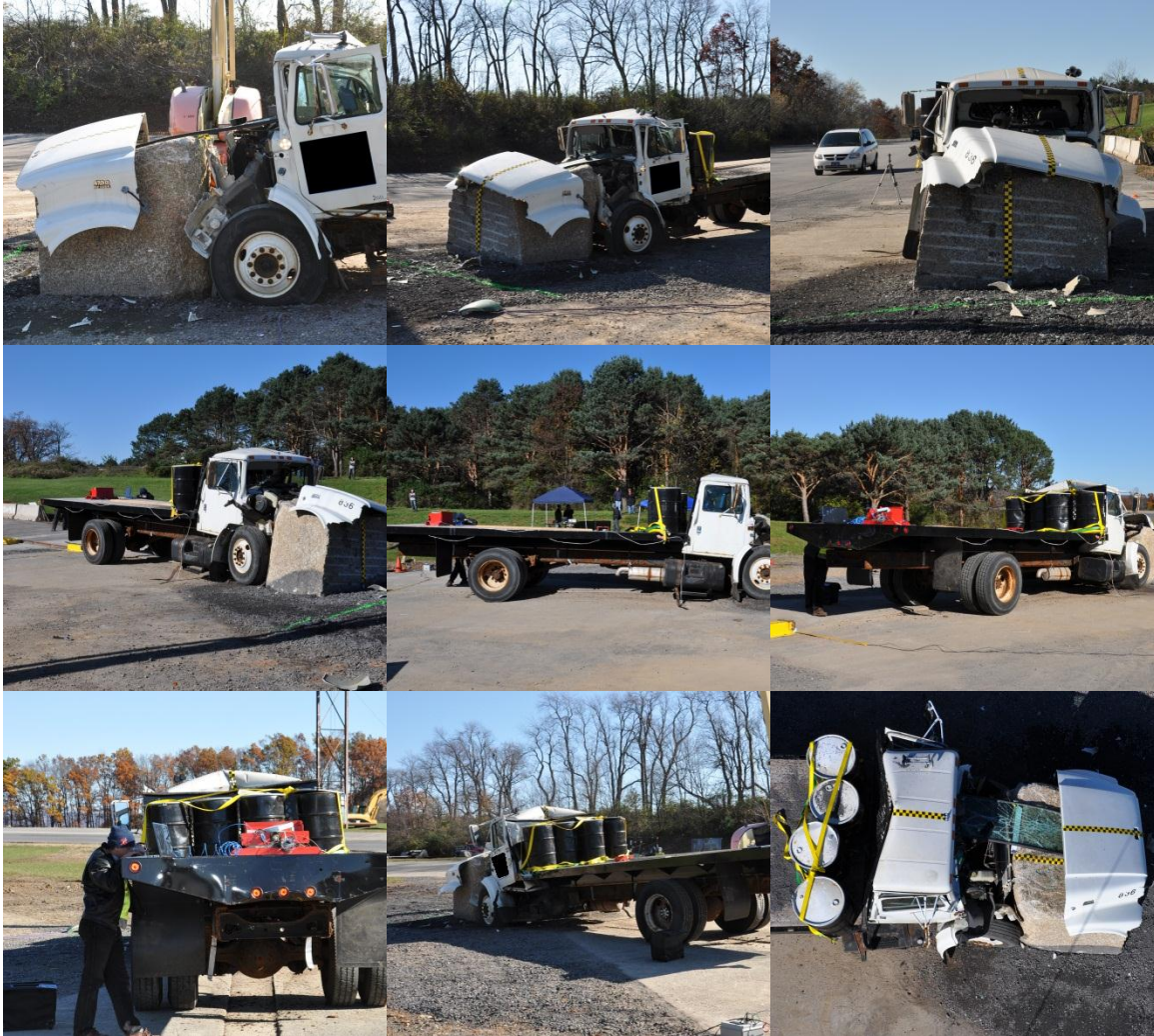
Figure 4-31. Post-test condition and location of the impact vehicle in BST-2
