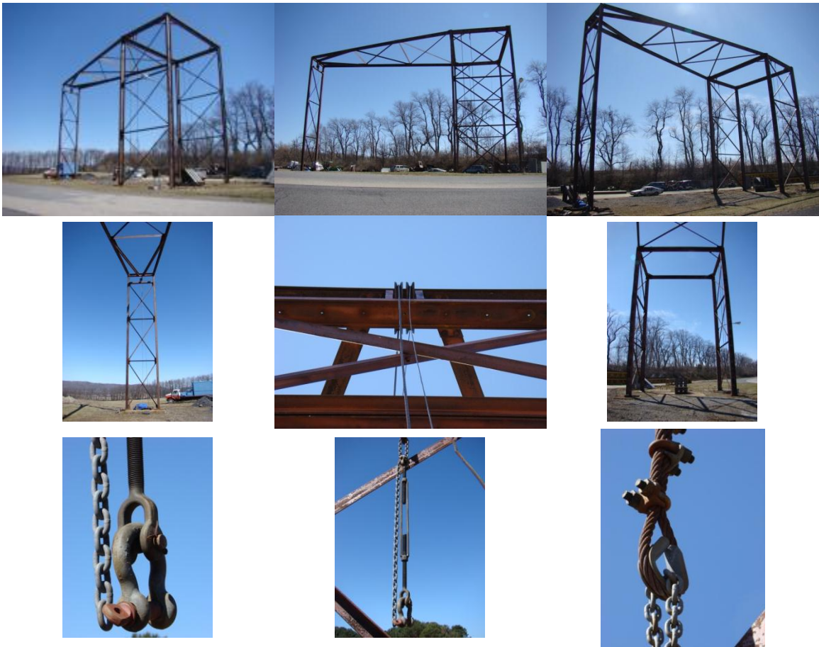
Figure 4-8. CRSI pendulum frame and components
