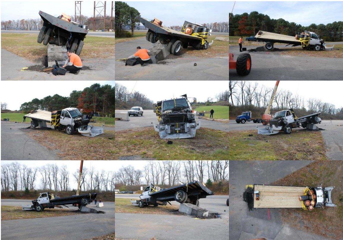
Figure 4-21. Post-test vehicle location in BST-1
