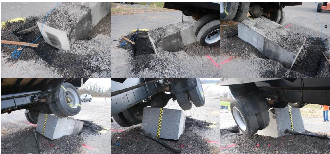
Figure 4-22. Post-test condition of ABG-01 in BST-1
