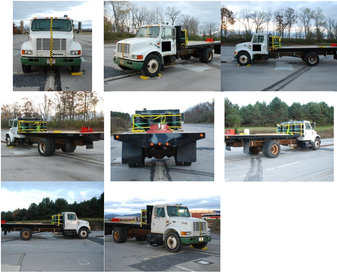
Figure 4-25. Pre-test condition of the impact vehicle in BST-2
