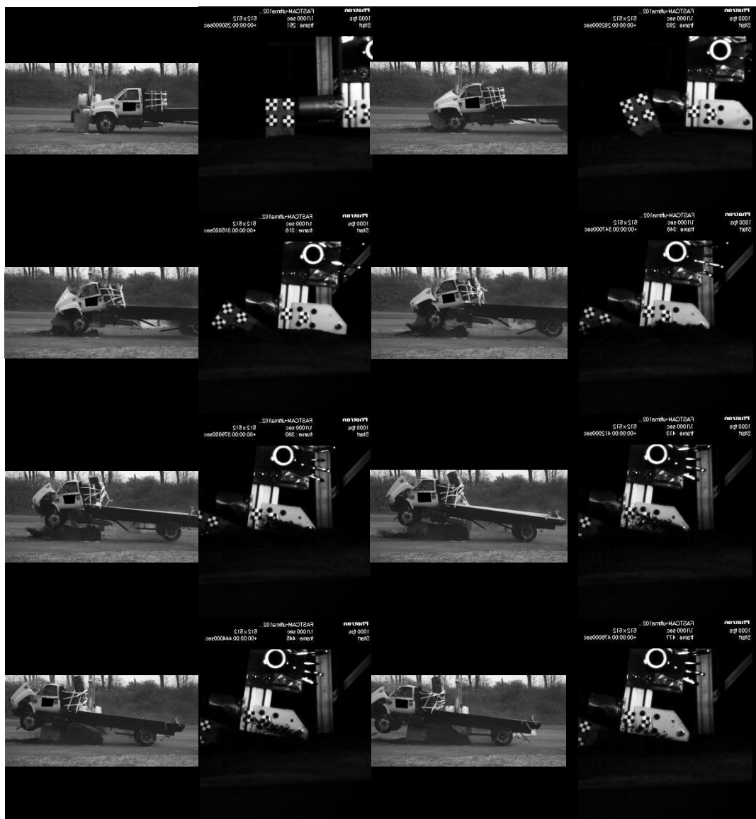
Figure 6-41. Comparison of high-speed image sequences from SSBST-1 and BST-1
