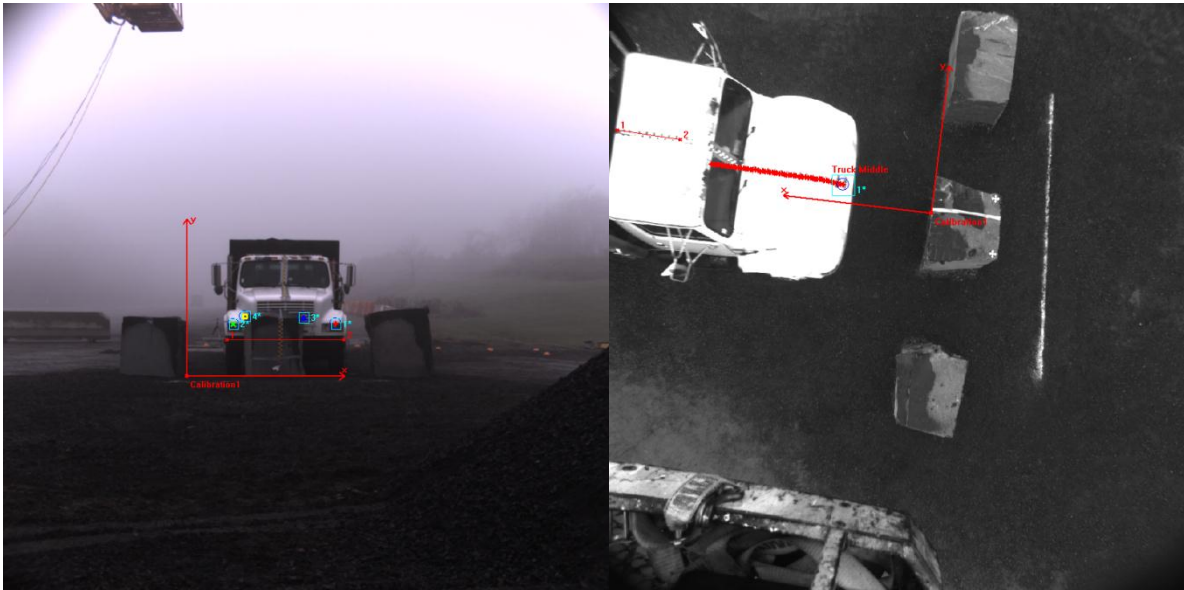
Figure 4-45. Location of impact vehicle centerline (left) and impact angle (right) in BFT-2
