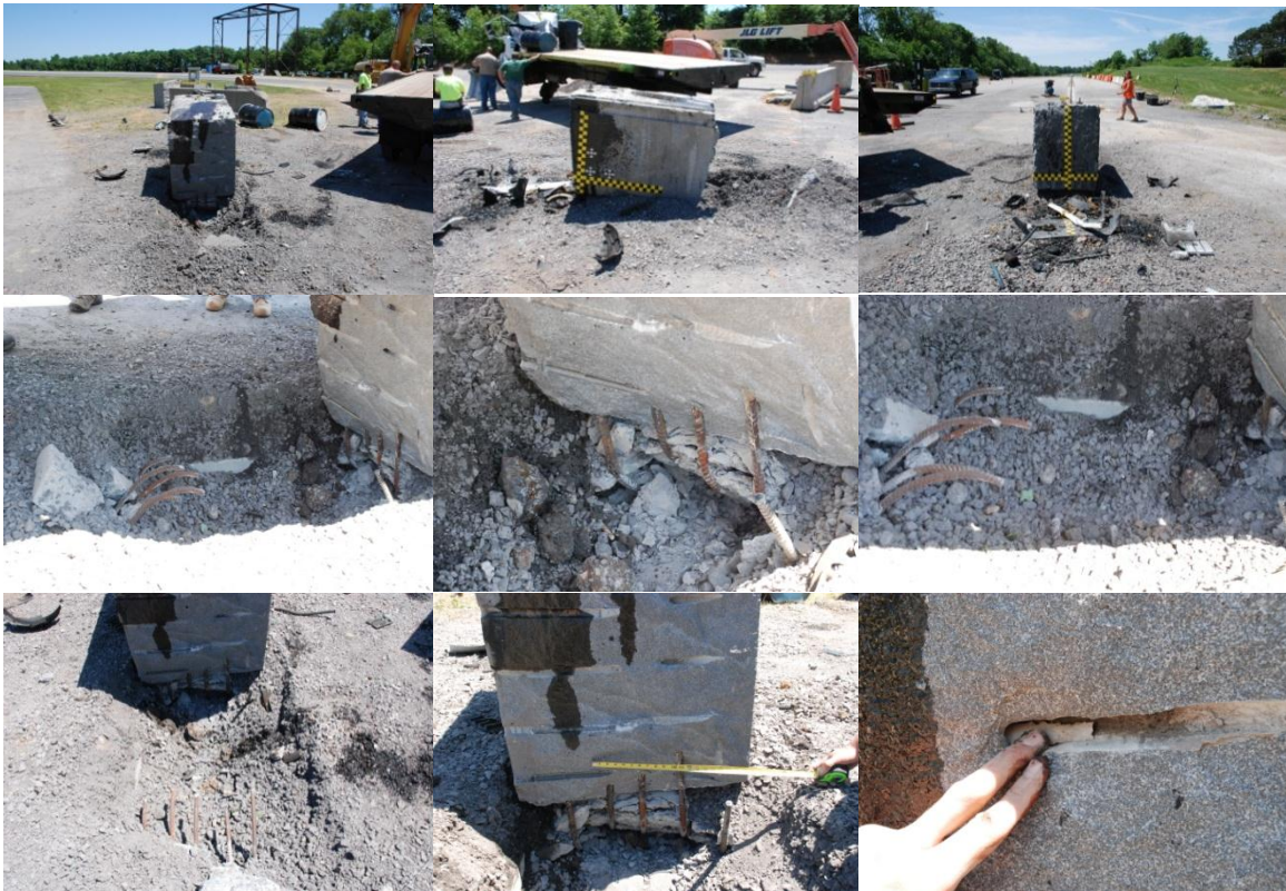
Figure 4-41. Post-test condition of ABG-02 in BFT-1
