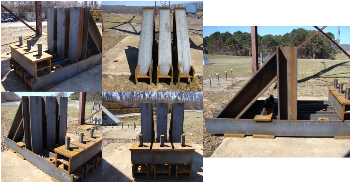
Figure 4-9. Skewbacks used in medium scale fracture testing
