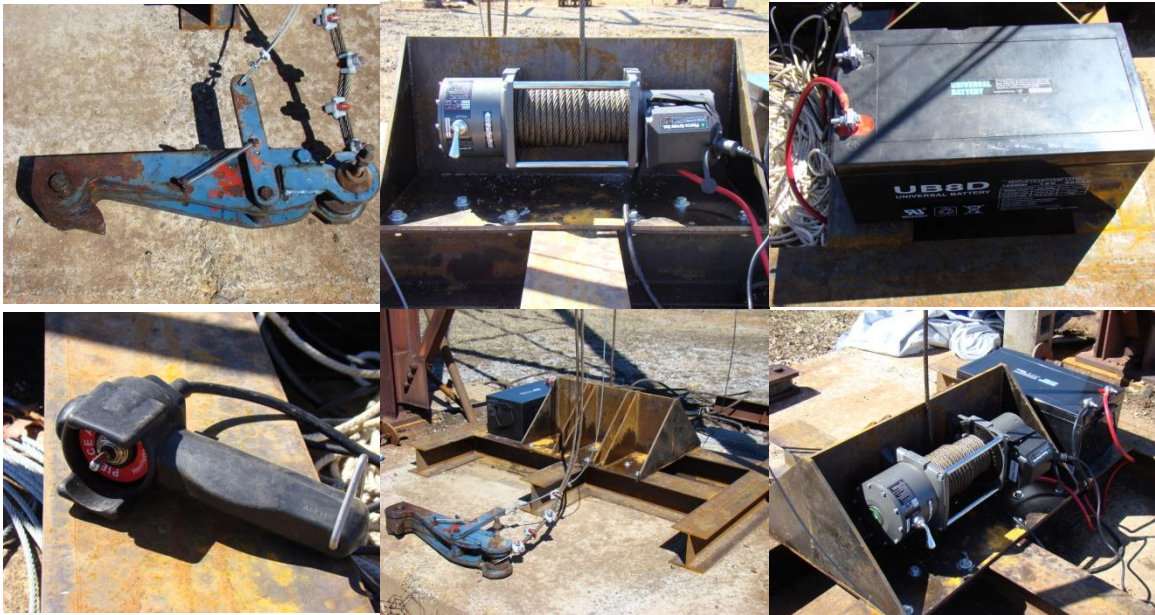
Figure 4-11. Impact sled raising system used in medium scale fracture testing
