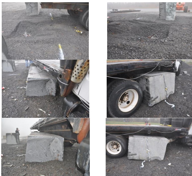
Figure 4-50. Post-test condition of ABG-03 in BFT-2
