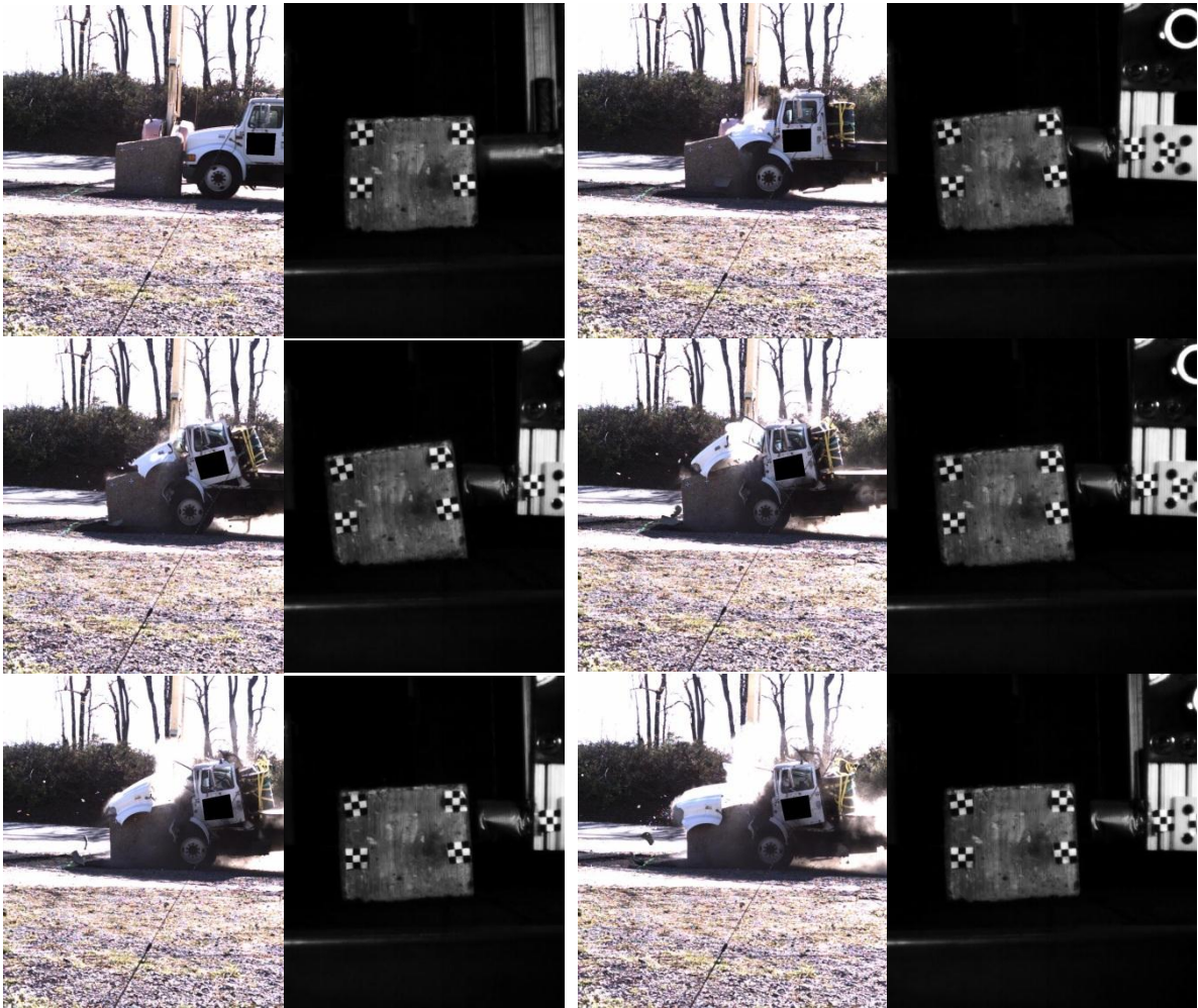
Figure 6-45. Comparison of high-speed image sequences from SSBST-2 and BST-2
