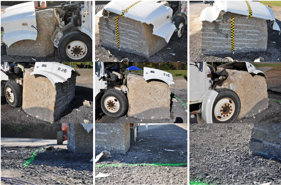
Figure 4-32. Post-test condition of RWG-01 in BST-2
