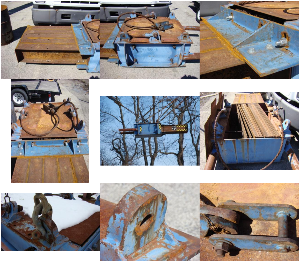
Figure 4-10. Detailed photographs of the impact sled used in medium scale crash tests
