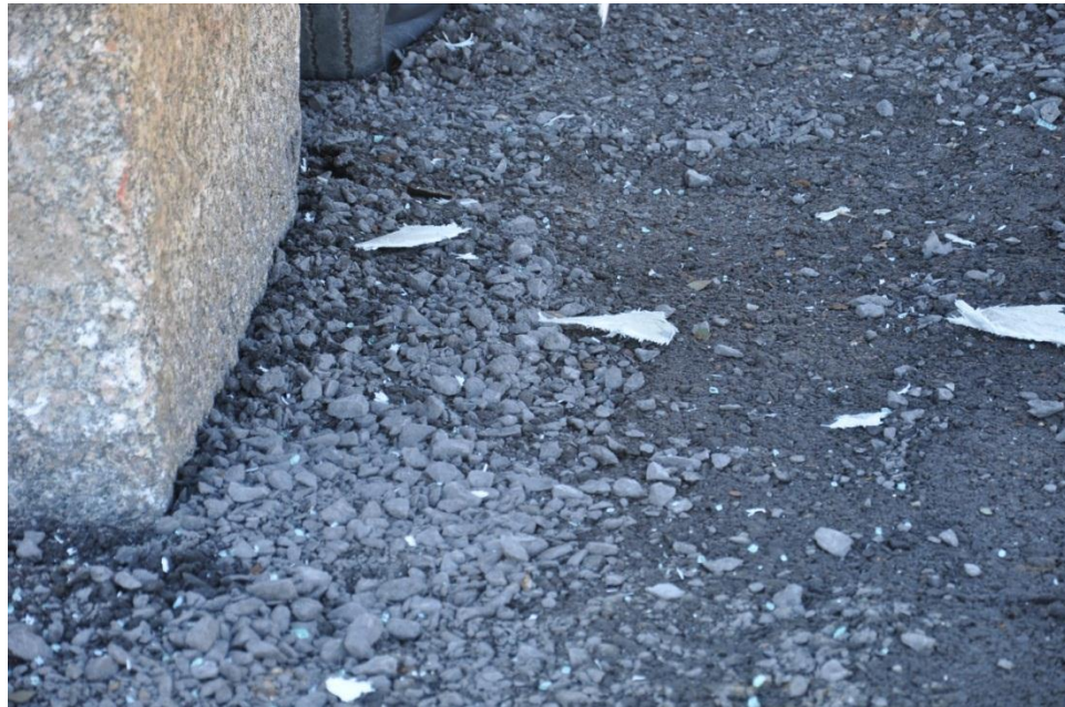
Figure 4-6. Modified 2A limestone gravel in compacted state
