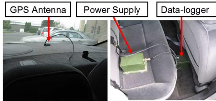
Figure 4.5: The sensors and data acquisition systems used in the experiments.
