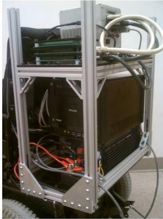
**Figure 3.3.** Hardware rack shown with xPC Target computer, ROS, and power architecture
