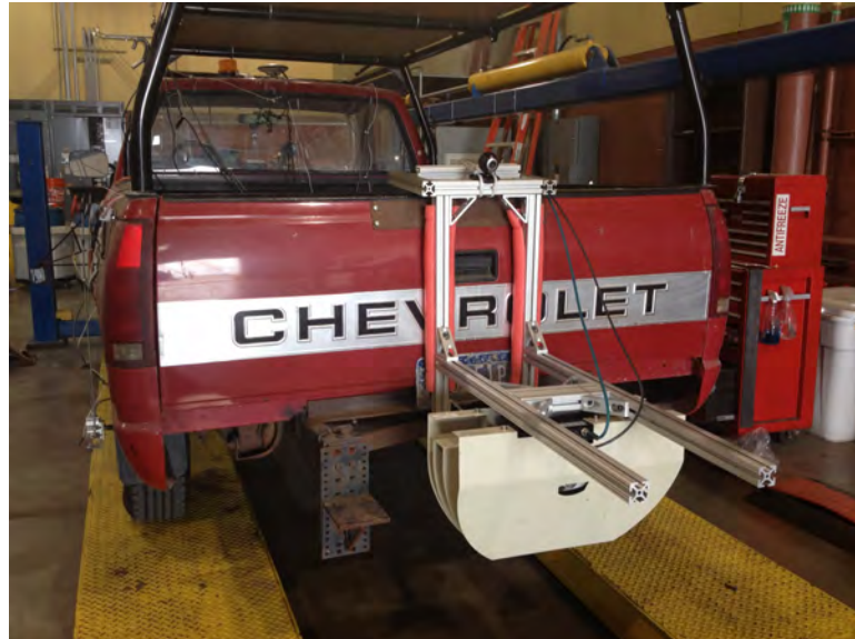
Figure 4.4. Lidar/GPS mapping rig on test vehicle
