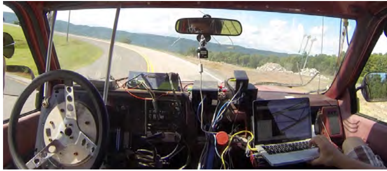
Figure 7.7. First-person view of 11\frac{m}{s} traversal of test track East turn under preview control/estimation
