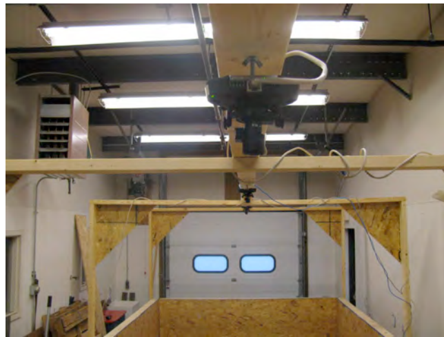
Figure 3-1: Cameras mounted to posts across support arches
