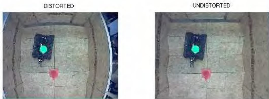
Figure 3-6: Distorted and undistorted images side-by-side
