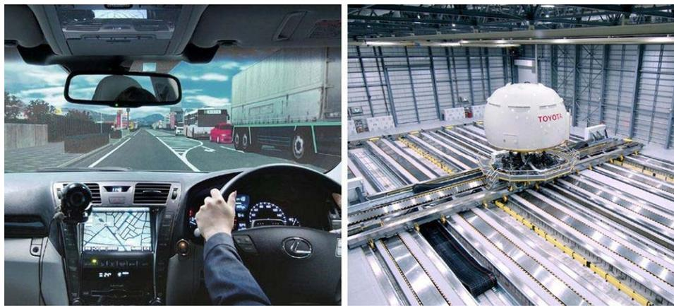
Figure 1-3. Interior (left) and motion platform (right) of Toyota's driving simulator [6]
