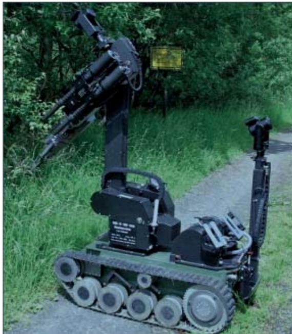
Figure 1-1. Telerobotic device for bomb disposal [1]
