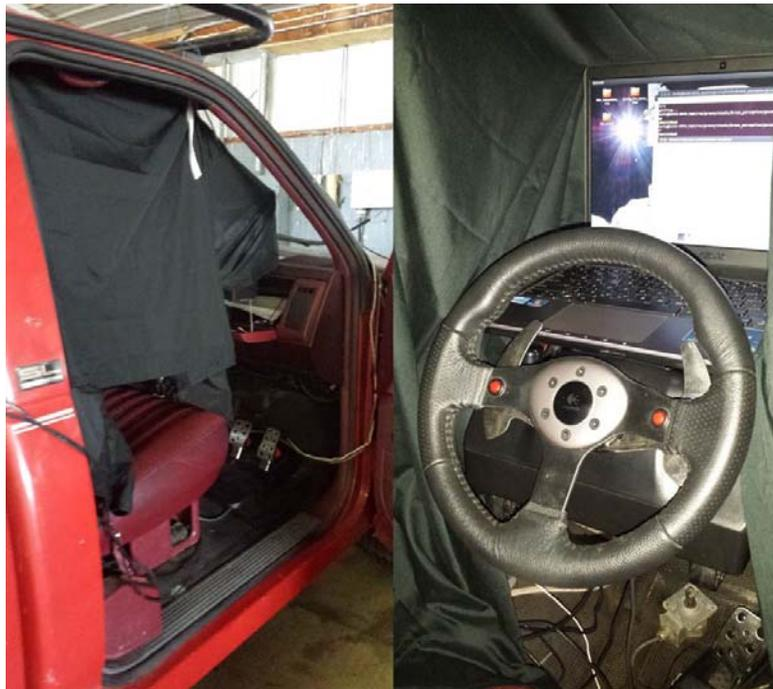
Figure 4-20. In-vehicle driving simulator
