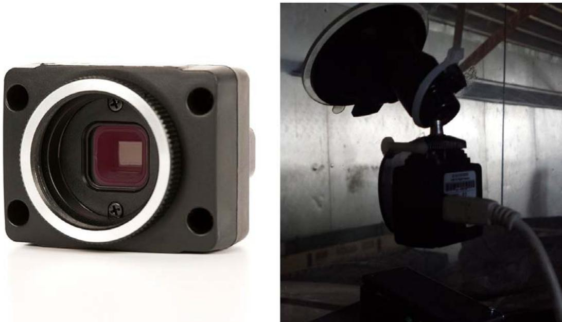
Figure 4-3. PointGrey Research Firefly MV USB 2.0 camera
