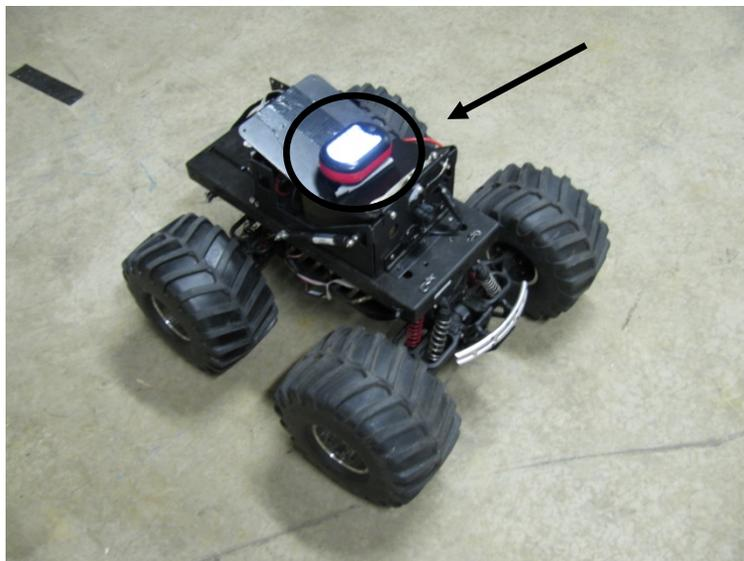
Figure 2-15: BomBot with LED fiducial
