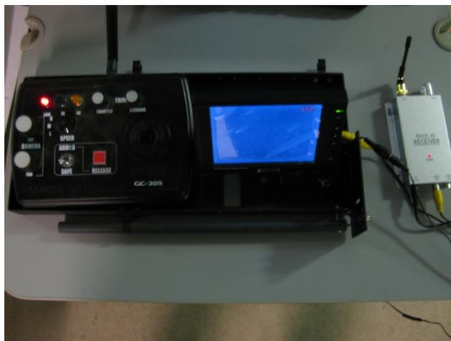
Figure 2-11: BomBot controller and teleoperation equipment
