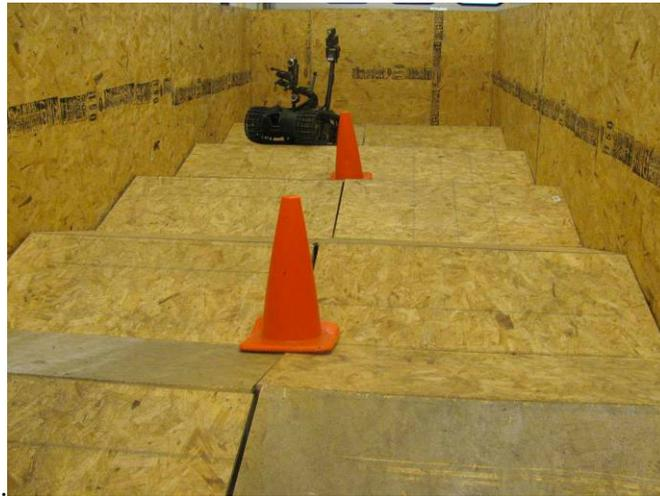
Figure 2-4: Continuous pitch/roll ramp setup
