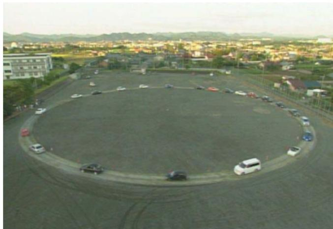
Figure 2.8: Experimental study of self-organized traffic jams performed by Sugiyama et al. [5]. A self-organized vehicle cluster can be seen in the top-right section of the image
